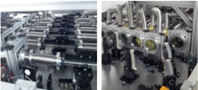
Image relay telescopes: high level of standardization
