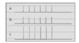
Two laser output synchronized to double the pulse energy and peak power, a) one laser output, b) a second laser output, and c) combined output.
