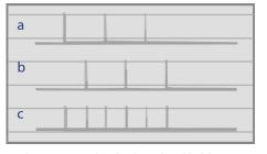
Two laser output combined with an adjustable delay to double the repetition rate of the pulse. a) one laser output, b) a second laser output with delay, and c) combined laser output.
