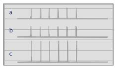
Two laser output synchronized to double the pulse energy and peak power, a) one laser output, b) a second laser output, and c) combined output.
